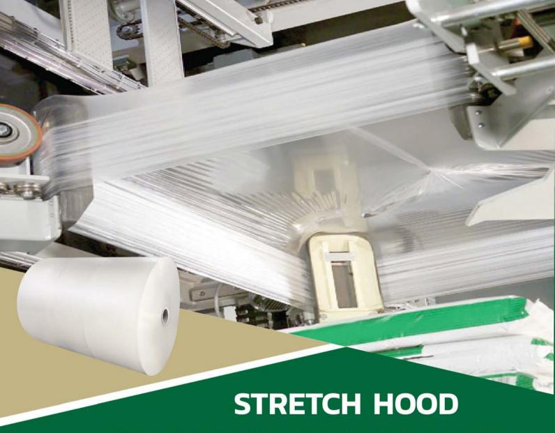
MMP Stretch Hood Film is a tube of film sealed at one end and stretched over a palletized load to secure the contents to the pallet. It provides load stability and abuse resistance. With five-sided protection, it ensures product stays dry and provide protection to all outdoor elements. The clear film also provides a good view of the packaged products.
