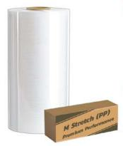
**Description**: This premium performance grade is formulated using the latest polymer technology. It has high film toughness and provides opportunities to use thinner film or higher pre-stretched levels to lower the cost per pallet wrapped. Total stretch level could be as high as 300% with higher film gauges. It is suitable for high speed automatic and semi automatic stretch wrappers.
